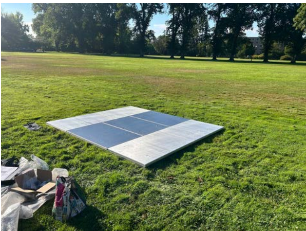
Figure 3. A 'fluidless' snow pillow assembled on the campus of Oregon State University.
