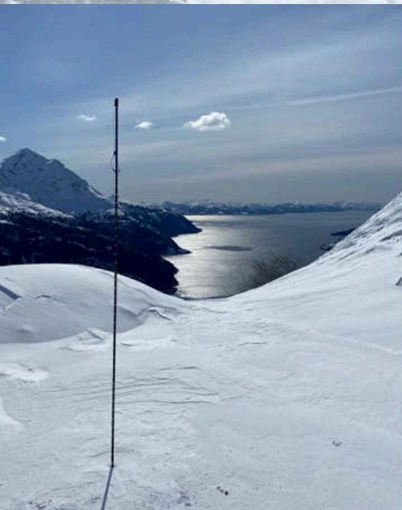
Figure 4. (Left) A snow probe is stuck into the snow to measure snow height, on April 7, 2021, above the landslide. (Right) An extracted snow core is measured and weighed to estimate snow water equivalent. In this photo taken during the field campaign on May 5, 2023, we verify that we reached the ground by seeing this "dirty bottom". Photos: Wikstrom Jones
