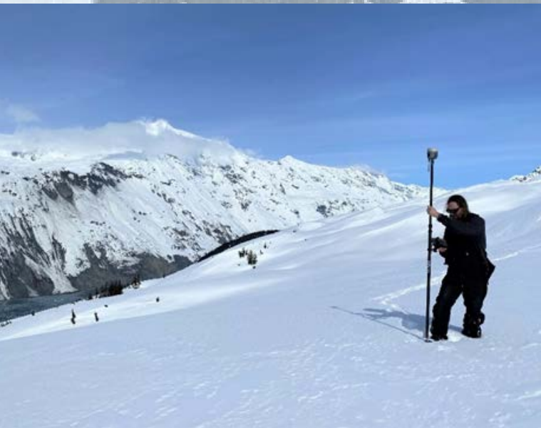
Figure 2. (Left) Ronald Daanen ( In memoriam ) collects ground control points on the east side, April 7, 2021, to use for lidar point cloud validation. Barry Arm landslide in the background. (Right) Location of GNSS base station supporting the lidar survey on May 5, 2023. Photos: Wikstrom Jones
