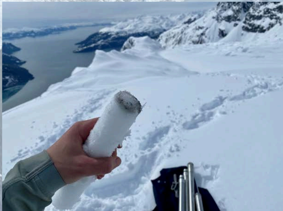
Figure 4. (Left) A snow probe is stuck into the snow to measure snow height, on April 7, 2021, above the landslide. (Right) An extracted snow core is measured and weighed to estimate snow water equivalent. In this photo taken during the field campaign on May 5, 2023, we verify that we reached the ground by seeing this "dirty bottom". Photos: Wikstrom Jones
