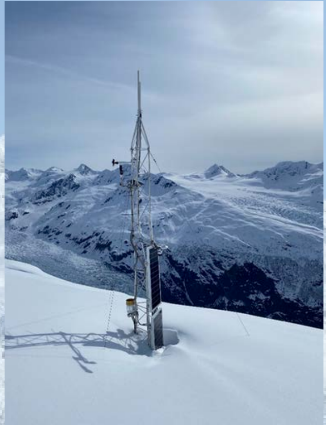
Figure 3. Snow height measured by a Campbell Scientific Sonic Ranger 50 at BAW above Landslide A.
