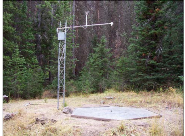
Figure 2. Example of a typical Snotel Telemetry station with a fluid-filled snow pillow on the ground.
