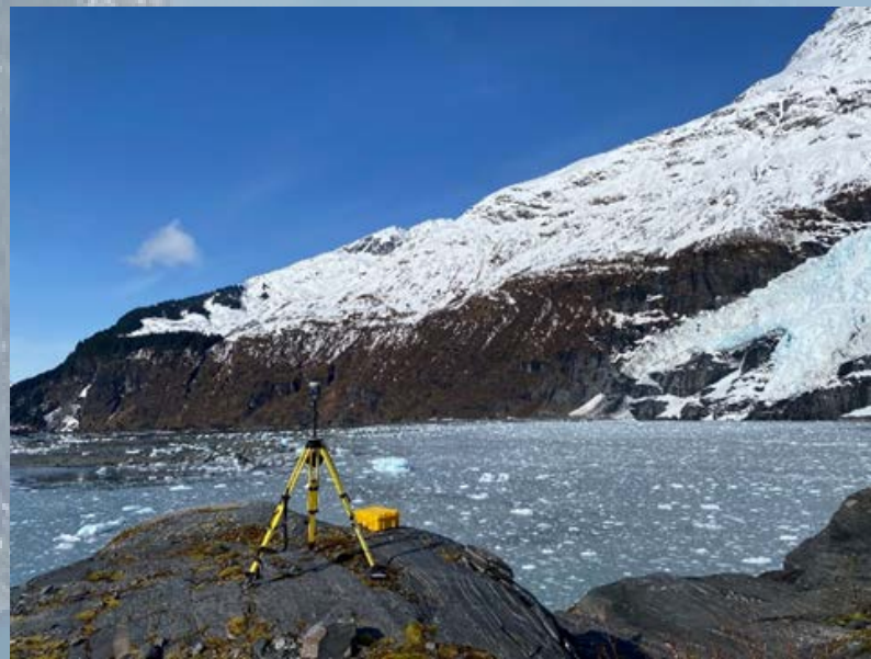
Figure 2. (Left) Ronald Daanen ( In memoriam ) collects ground control points on the east side, April 7, 2021, to use for lidar point cloud validation. Barry Arm landslide in the background. (Right) Location of GNSS base station supporting the lidar survey on May 5, 2023. Photos: Wikstrom Jones
